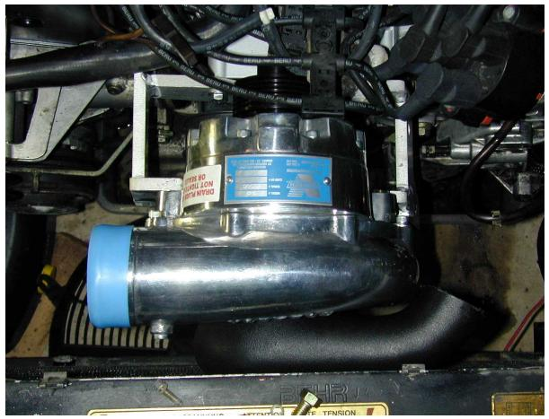
and bolt in place with the bolts and lock washers as listed in the parts list. Connect oil return hose from underside of blower (accessible from top of car, on passengers' side) and clamp in place. Route oil return line around belts and into position and secure to dipstick dowel at base, & clamp.
