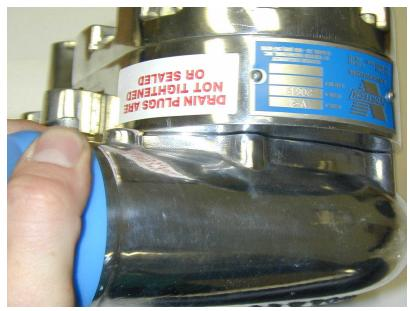
(Loosen the 6 allen screws and banana washers and rotate blower housing to match photo above, replace screws and banana washers when complete)
