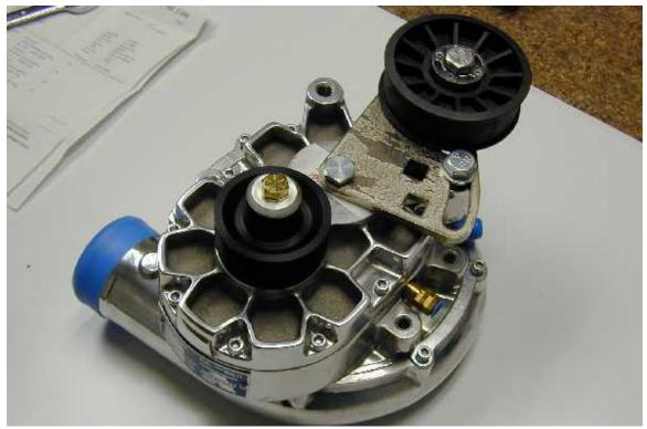
(Assembled supercharger, pulley, and tensioner, with uncorrected center pivot bolt penetrating white sticker, it should be a set-screw instead
