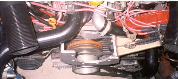
slip blower assembly into bracket (**photo**), removing your upper radiator grommets will help you achieve the leverage necessary
