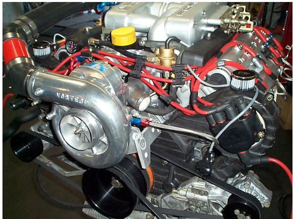
**Overview:** This supercharger kit was designed for the 32-valve 928 cars, from 1985-1995, though should fit the earlier '80-84 US cars with little modification, and will fit the '84-'86 euro efi cars with no mofifications. **Warning:** Different pulleys will be needed for the earlier cars ('80-'84) to prevent the supercharger kits from making too much boost on the lower horsepower'd cars. Vortech will assist you with proper pulley and FMU selecting (see back of manual)
