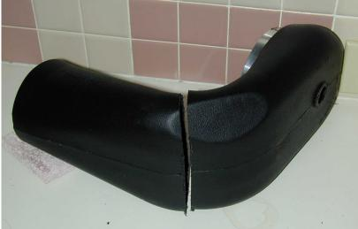
(Cut inlet elbow exactly as shown, notice that the 1" dia. Bung has been cut off, this hold needs to be patched/plastic welded) before installation.)
