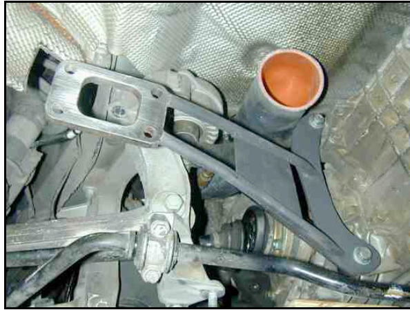
Photo 7.1. Turbo Bracket installed.
