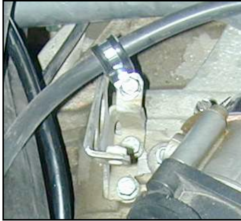
Photo 16.1. Vacuum-Boost Hose clamp eye bracket location.
