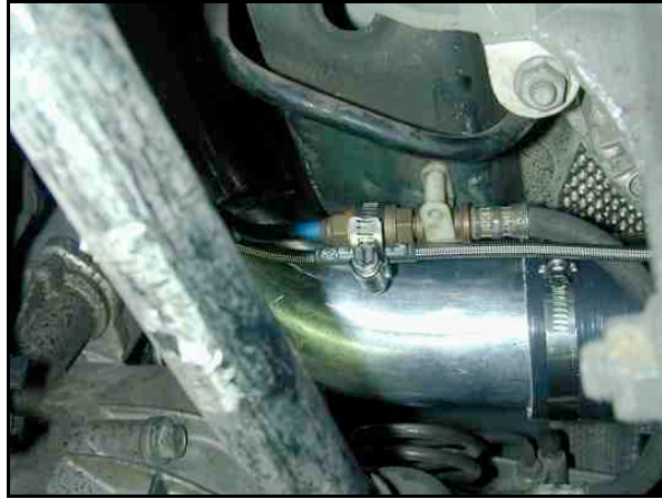
Photo 8.2. -3AN Oil line secured.
