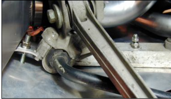
Photo 17.6. Intercooler Heatshield rear and center mounts.
