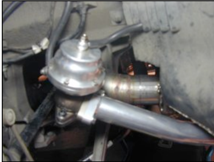
Photo 16.5. Wastegate Pipe installed.
