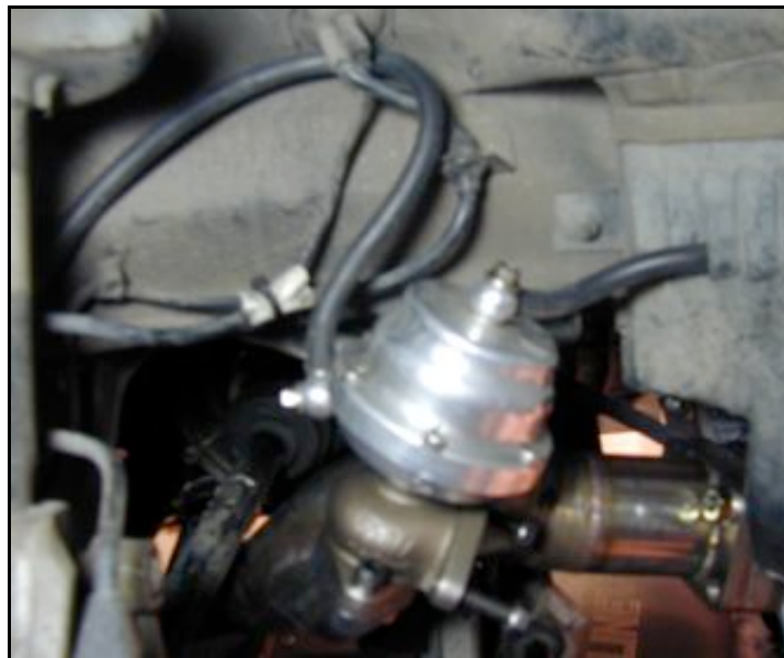
Photo 16.4. Wastegate mounted with hoses attached.
