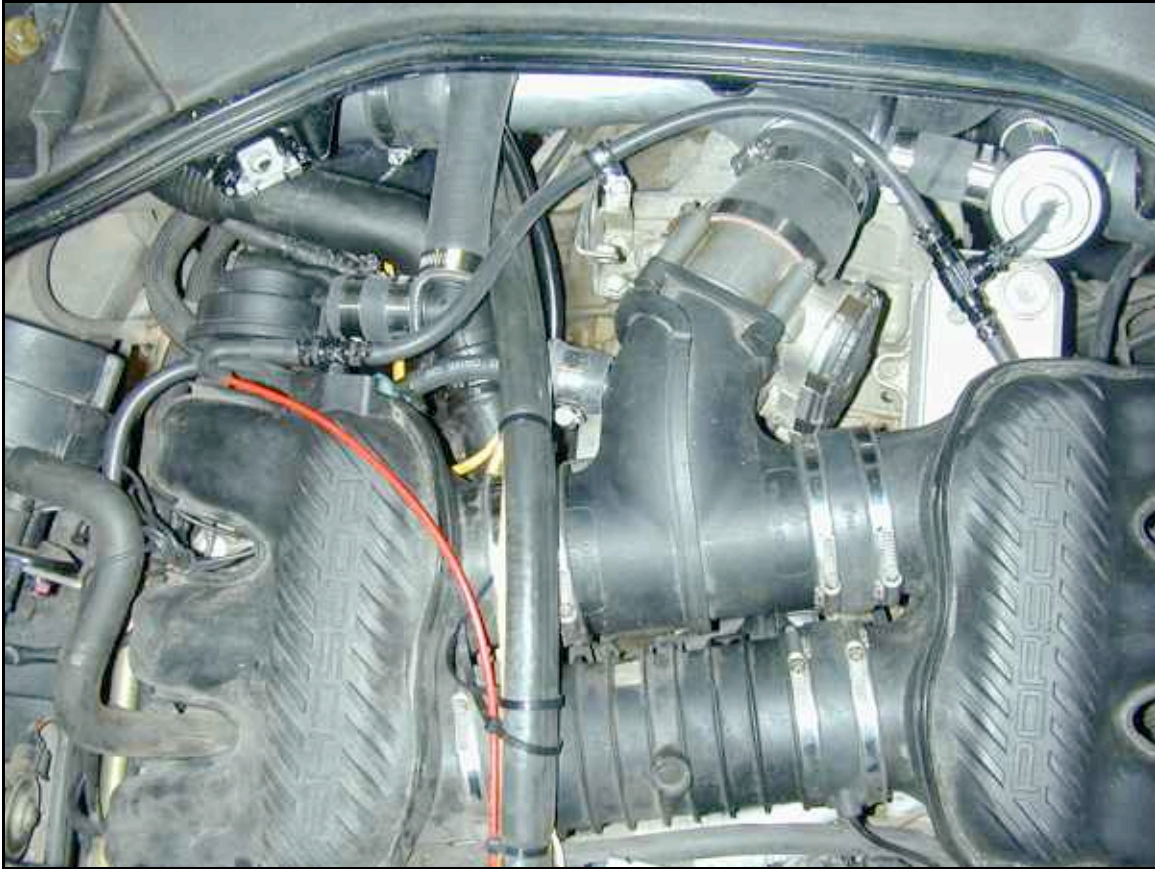
Photo 16.0. Vacuum-Boost Hose installed (top view).
