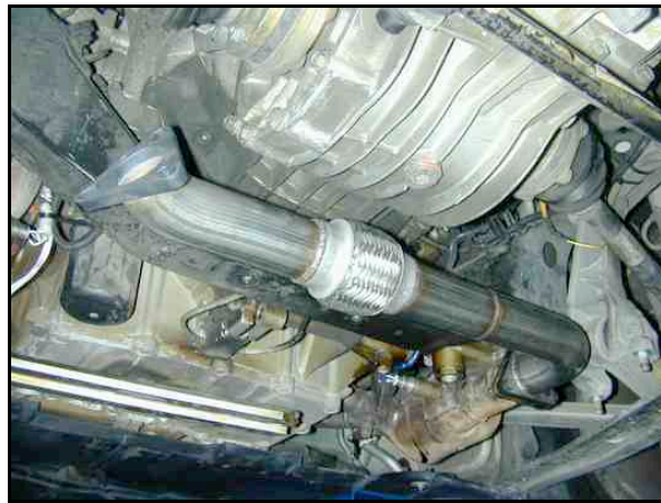
Photo 7.2. Right side exhaust pipe installed.
