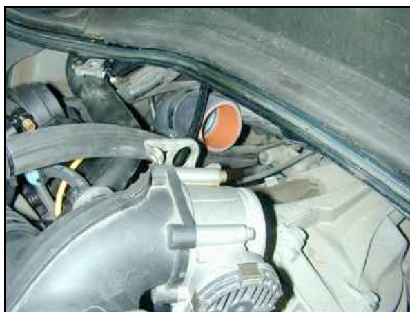
Photo 14.0. Top of Boostpipe #2 in position.
