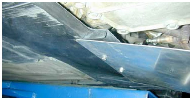
Photo 17.3. Intercooler Heatshield front fasteners installed.
