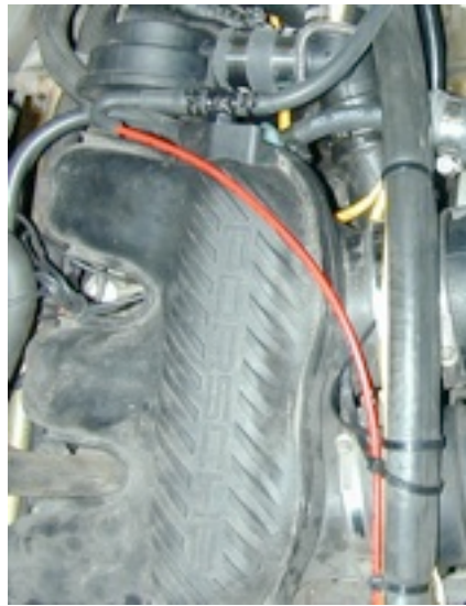
Photo 19.0. Boost Gauge vacuum line routing.
