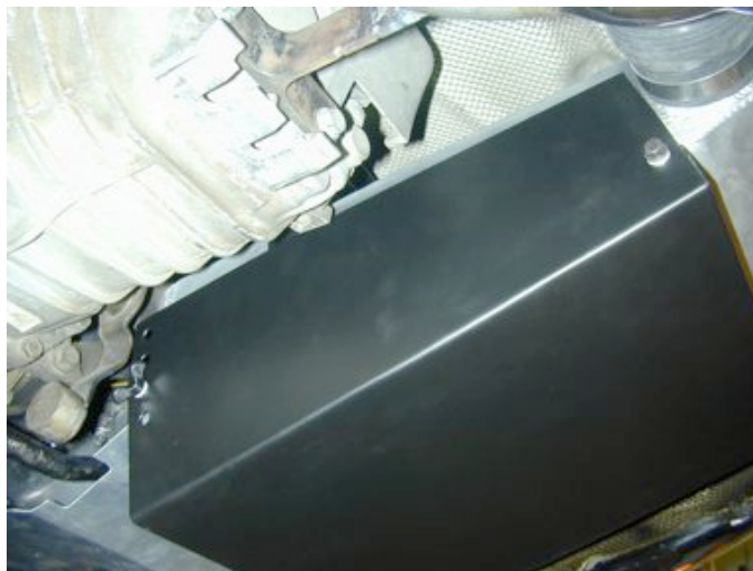
Photo 18.2. Intercooler Air-duct installed.
