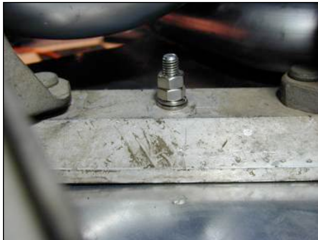
Photo 17.5. Intercooler Heatshield center fastener installed.
