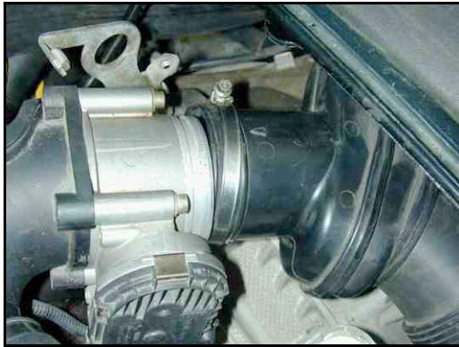
Photos 3.0-3.1. Intake clamps loosened.
