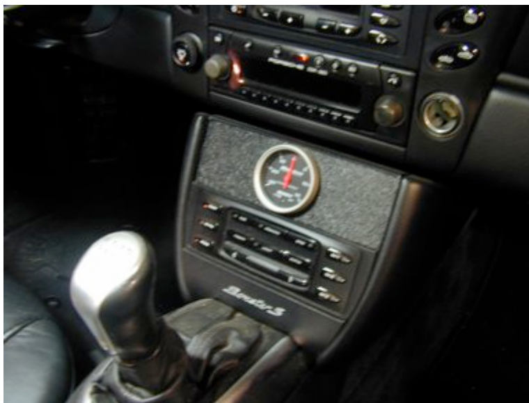
Photo 19.2. Suggested Boost Gauge installation.
