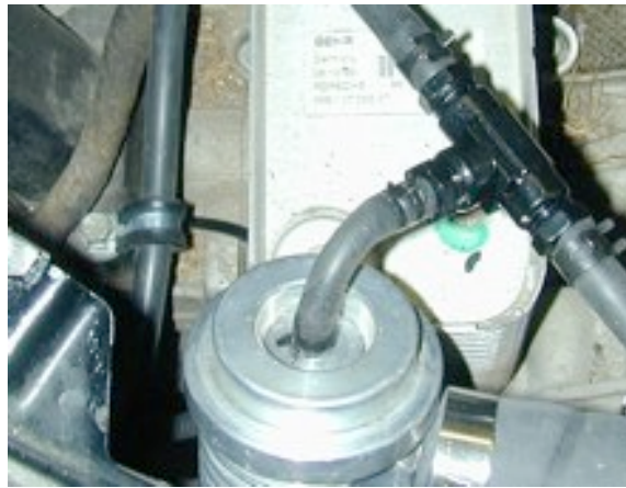
Photo 16.2. Vacuum-Boost Hose clamp plenum bolt location.
