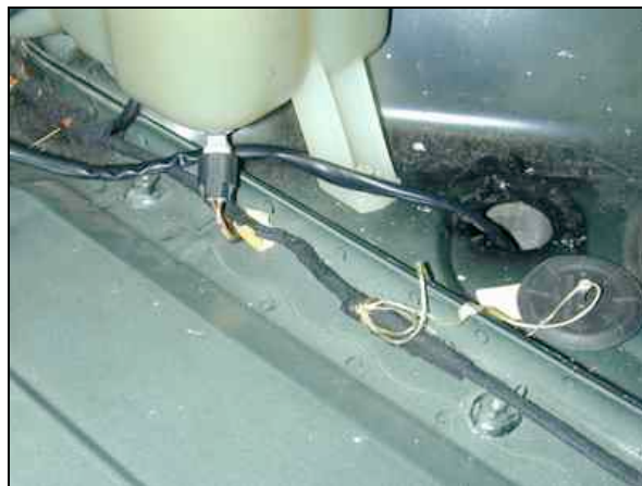
Photo 11.5. Harness dropped through trunk hole.
