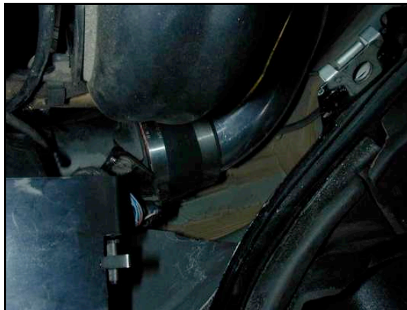
Photo 6.5. Intake Pipe installed on MAF.
