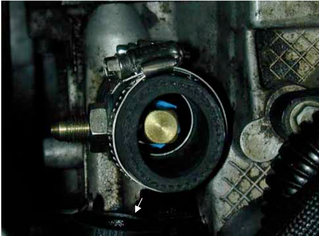
Photo 9.4. Oil return assembly installed with loose clamps.
