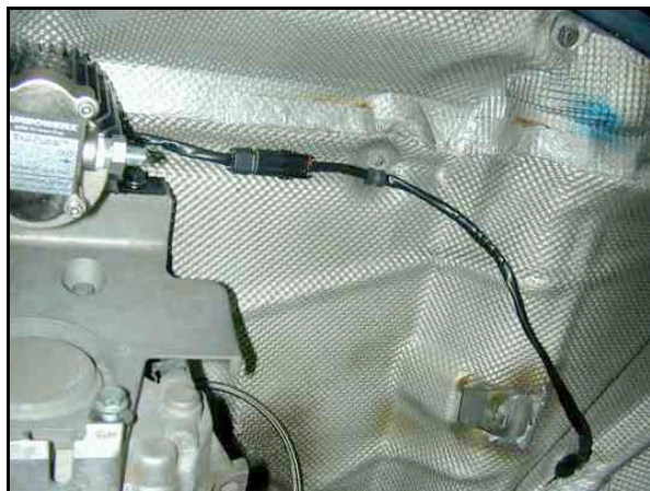
Photo 11.10. Harness connected to Scavenge Pump.
