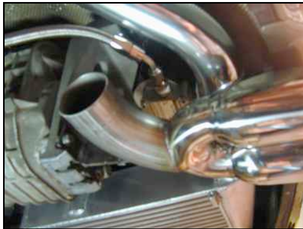
Photo 13.4. Exhaust tip mounted.
