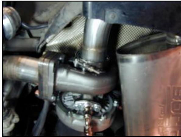
Photo 13.4. Muffler mounted on turbo with V-Band clamp.
