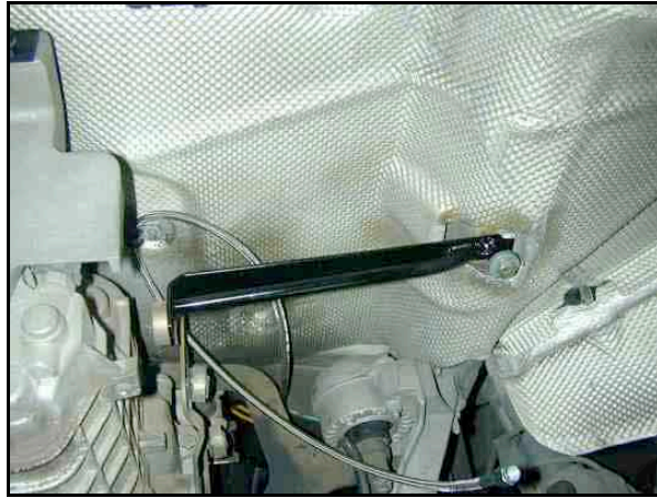
Photo 10.2. Intercooler Bracket mounted.
