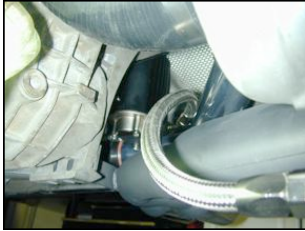
Photo 13.7. -6AN Turbo Oil Drain Hose clearance.
