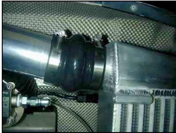
Photo 13.1. Boostpipe #1 hump hose installed.
