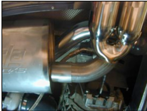
Photo 13.5. Muffler mated to tip.
