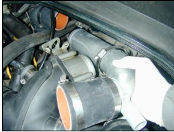
Photo 14.4. Boostpipe #3 ready to install.
