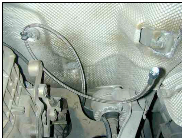
Photo 10.1. -4AN Oil Line looped through clamp.
