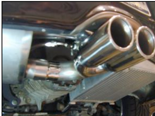
Photo 13.5. Muffler mated to tip.
