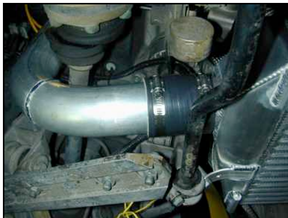
Photo 14.3. Boostpipe #2 bottom installed.
