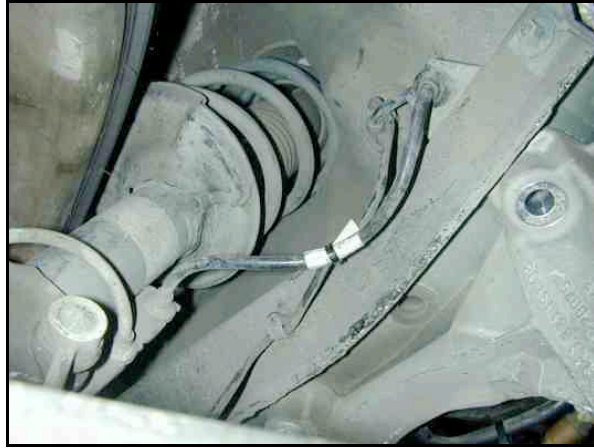
Photo 7.3. ABS cable secured with tie-wrap.
