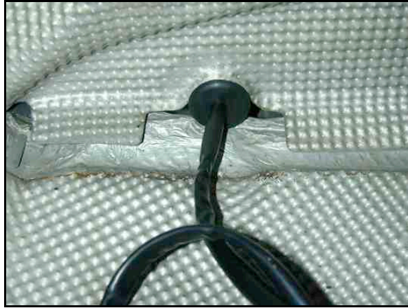
Photo 11.8. Harness grommet installed.
