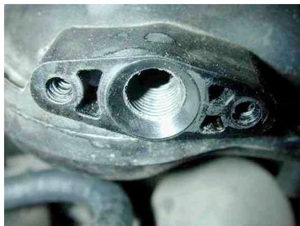
Photo 1.6 1/4" NPT tapped thread.
