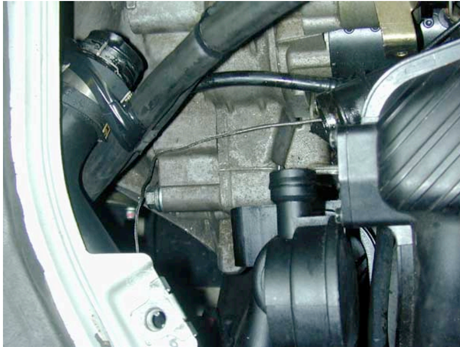
Photo 9.0. Temporarily securing plastic oil filler tube.
