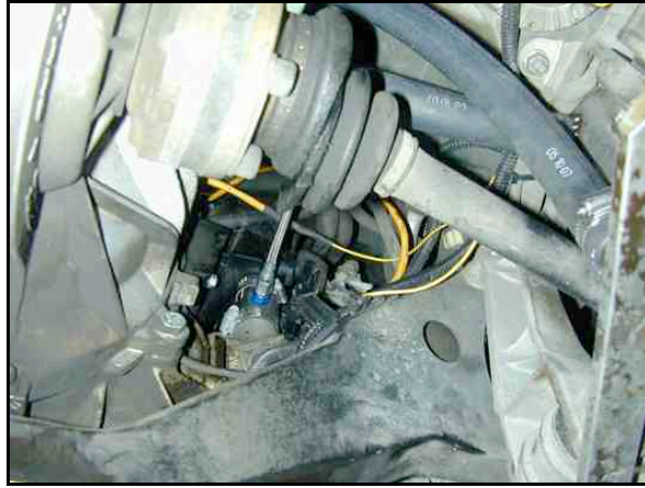
Photo 9.7. Oil Return Assembly installed.
