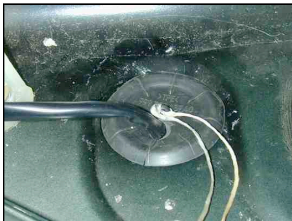
Photo 11.7. Harness inserted through modified plug cap.
