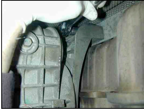
Photo 5.4. Ratchet on muffler support bolt.
