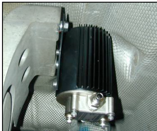
Photo 10.0. Scavenge Pump mounted.
