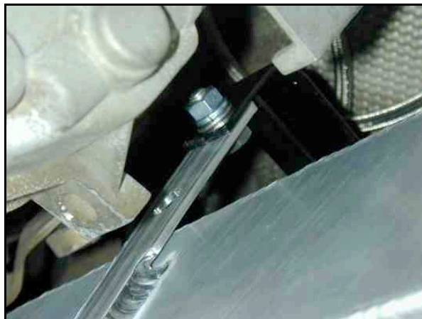
Photo 12.2. Intercooler top support fastener.
