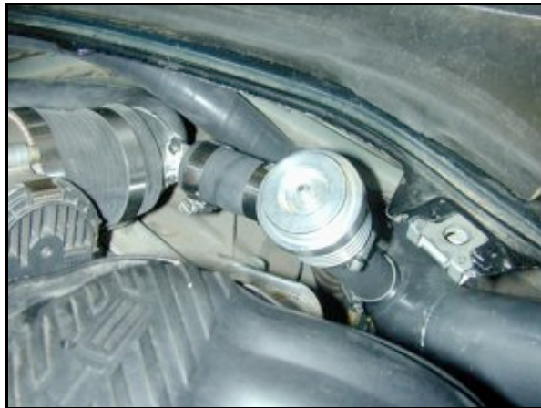
Photo 15.3. Recirculation Valve Assembly installed.
