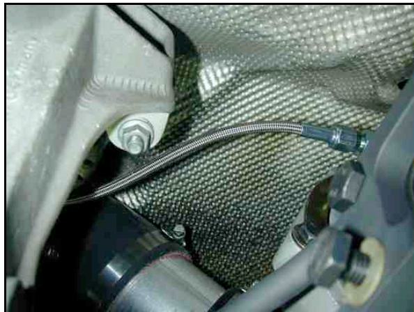
Photo 8.3. -3AN Oil line connected to turbo.
