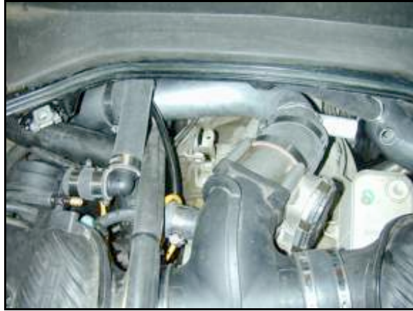
Photo 15.1. Crankcase Hose installed.
