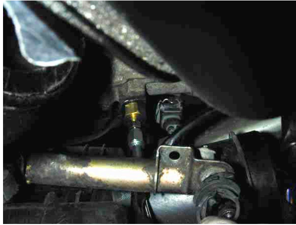
Photo 1.2. -3AN adapter and -3AN oil line installed.
