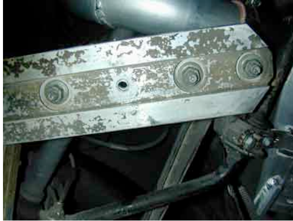
Photo 17.0. Location of drilled hole for heatshield center mounting point.
