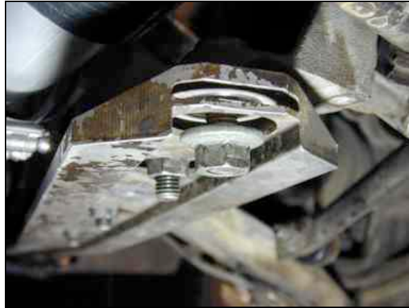
Photo 18.0. Nut flush with stud for stud removal.
