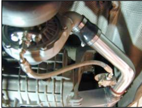
Photo 13.3. -6AN Turbo Oil Drain Hose installed.
