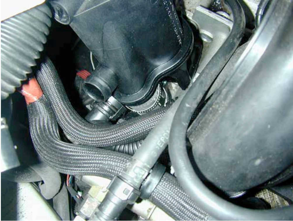
Photo 9.5. Air-oil separator during installation.
